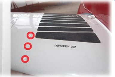
Investigation of riveted joints of the two-seat Zlin Z-142 trainer aircraft using the eddy current method using a matrix arrangement of measuring elements (Eddy Current Array, ECA)
