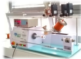
Numerically controlled single-spindle winding machine Ingrid West Machinery, type WH-751 for coils production
