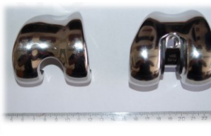
Standards of biocompatible prosthetic replacements for the investigation of electrically conductive biomaterial structures: part of a total hip joint endoprosthesis of a child made of Ti-Al-V alloy (left), a functional part of a knee joint made of stainless austenitic steel (center) and part of an adult hip joint endoprosthesis made of stainless austenitic steel (right)
