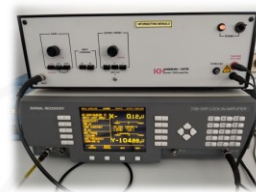
Lock-in amplifier Signal Recovery DSP 7280 and wide-band power amplifier Krohn-Hite 7500
